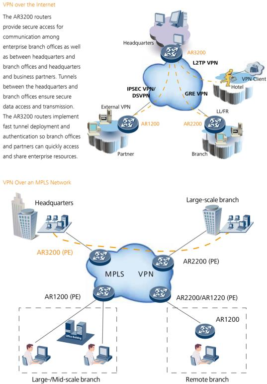
The AR3200 routers are well suited to serve as PEs in the headquarters office of a large enterprise. The MPLS L3 VPN segregates services by type. The AR3200 routers feature flexible deployment, fast distribution, and secure transmission of VPN services, as well as supporting enterprise service operation over networks.
