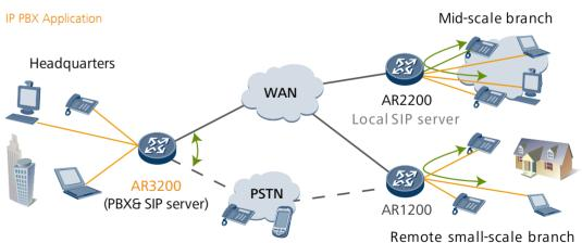
To improve communication efficiency, all AR routers include a built-in PBX. This feature supports the enterprise main number, Interactive Voice Response (IVR), and bill query functions. An AR1200 or an AR2200 router can be located in a branch office to provide the intelligent dialing feature.
