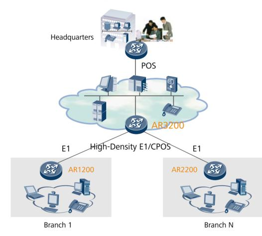
AR3200 series enterprise routers support the rich interface cards, including high-density E1, CPOS, POS interface cards and so on, to meet the convergence access requirements in the various branches and headquarters. Multiple enterprise small branches connected by E1 uplink to the aggregation layer routers. The aggregation routers use high-density the E1 boards or CPOS to converged access, and then through the POS uplink to connect the high-end router of the core network.
