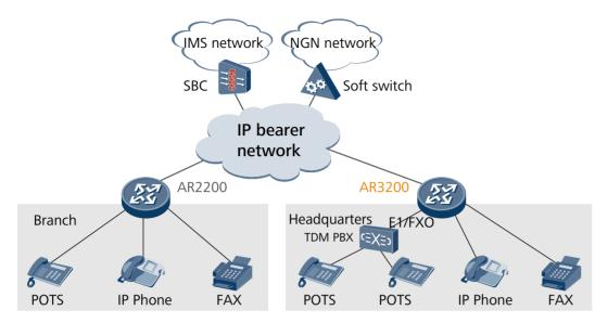
The AR3200 routers integrate voice, fax, and IP services. For enterprise users, the AR3200 routers serve as a SIP access gateway for the headquarters office, transforming phone signals into VoIP signals. The AR3200 routers uplink interfaces connect to the IP Multimedia Subsystem (IMS) or Next Generation Network (NGN) to allow any media, including phones, handsets, and computers, to communicate at any time.
