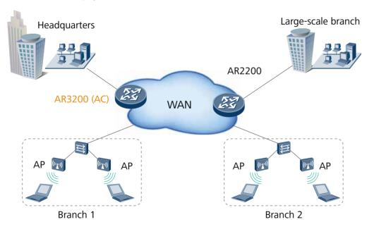
The AR3200 routers integrate AC (Access Controller) functionality, which can manage the wireless AP (Access Point) in wireless LAN. AR3200 supports rich certification and flexible user access control, which can provide security access guarantee for Wi-Fi users. The rich wireless capabilities integrated in one device, this can realize centralized management of wired and wireless networks, to meet the requirements of different scale enterprises networks.
